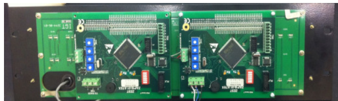
Shown - Dual microphone and twin transceiver A + B N+2 execution for mission critical fault tolerant PAGA applications.
