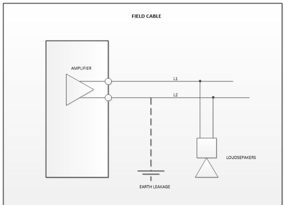
Earth leakage detection is independent of the loudspeaker circuit topology and operates in the same way for loop, radial, star or 'tree and branch' wired networks. Earth leakage current flow is supervised on both loudspeaker line conductors and the detection circuit can resolve up to 68kOhm between either conductor and dirty earth.
