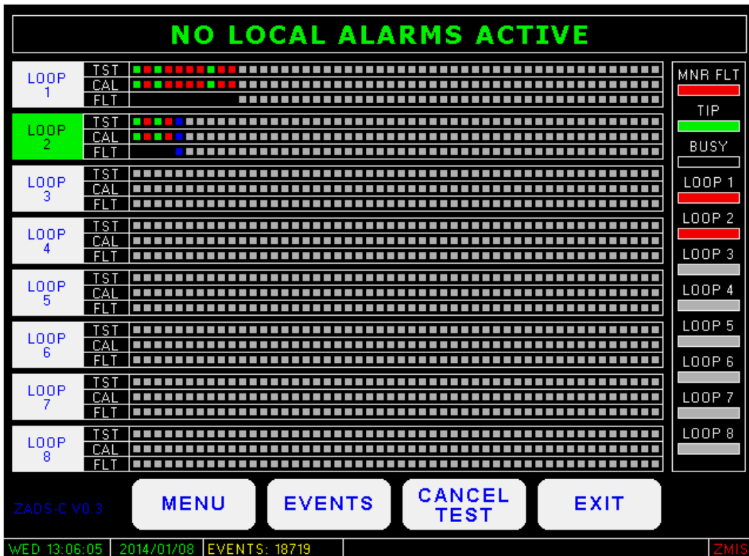
Comprehensive interface for the configuration, testing and status reporting of individual loudspeaker devices.
