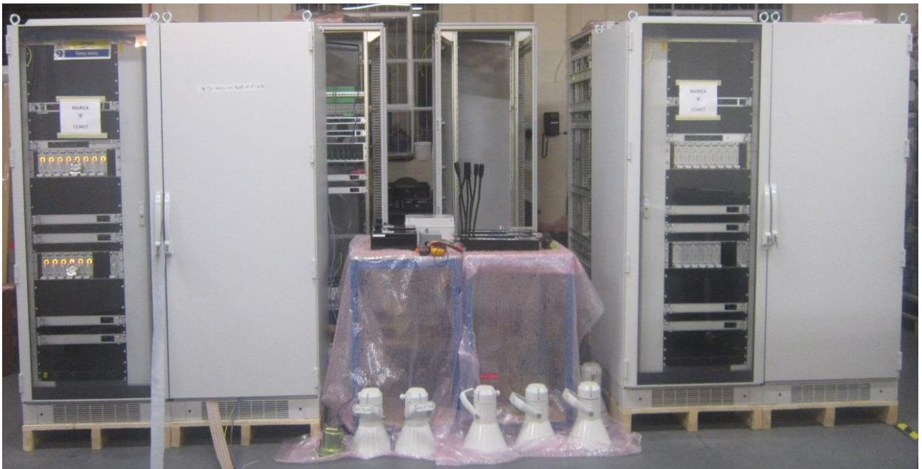
*Typical A+B ZEST PAGA system undergoing FAT in our factory. Note the two identical panels which each drive associated A+B field equipment to ensure no common mode failure possibility.*
