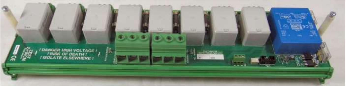
Photo above shows DIN rail mount Z+1 ACM Module, note the use of multiple switching elements which improve security. Each power circuit of the Z+1 ACM Module has dedicated multiple changeover facilities eliminating the **single point of failure** introduced when using a single change-over contactor. The switching environment is also sealed ensuring long through-life reliability in this highly critical component.
