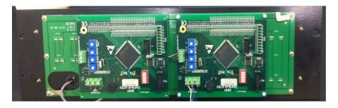
Above rear view of AP100-01 shows duplicated transceivers fitted for secure N + 1 or A + B applications
