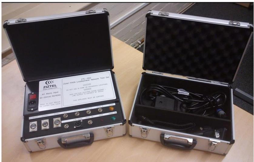
ZTL350 set comprises of two portable carry cases, test set and cable set
