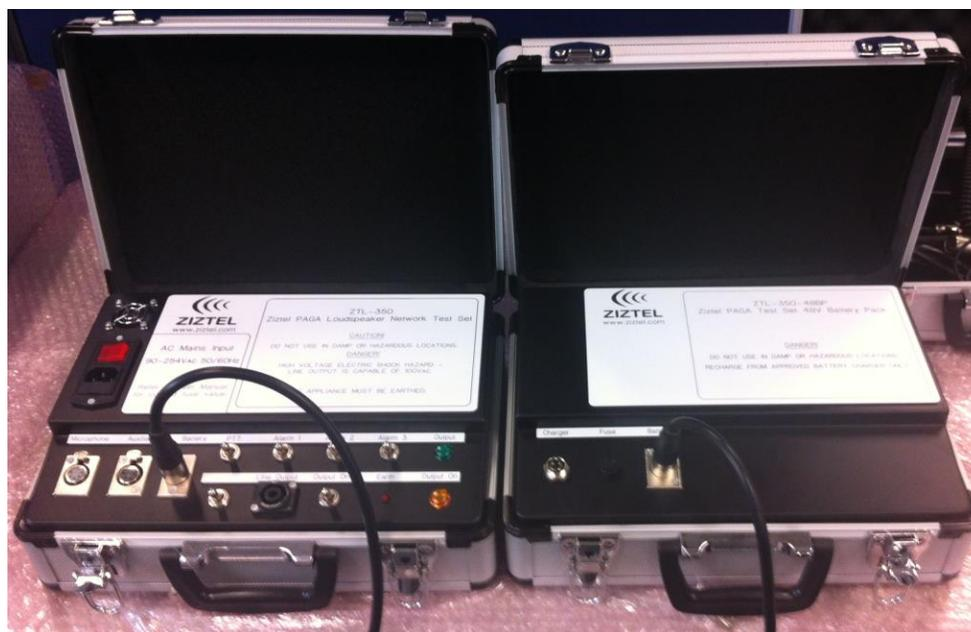
The above photo shows the ZTL350 and optional ZTL350B secondary carry case which incorporates a no break battery pack enabling operation in the absence of site AC mains supply. Battery autonomy is 1 hour operation at full power for tick tone testing and speech. Sites usually procure two battery packs, cycling one ‘on charge’ and ‘one in use’ to enable continuous PAGA testing.
