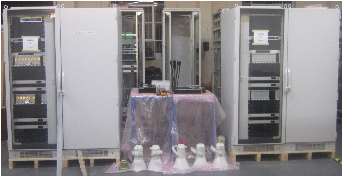
Typical view of an A+B ZEST PAGA system undergoing FAT in our factory. Note the two identical panels which each drive associated A+B field equipment to ensure no common mode failure possibility.
