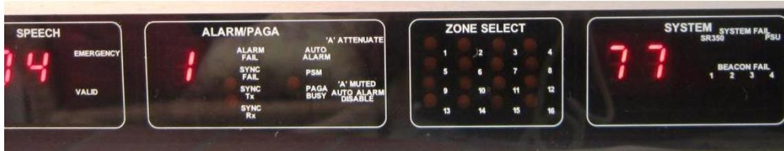
*ZXM32 is fitted within the Zitel ZEST ZX100 management processor. Message status is described by numerical output fitted to the fascia of the ZX100*
