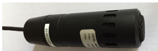
The rugged ATEX certified MG600 microphone transducer as used in all variants of the MG600 Ex i
