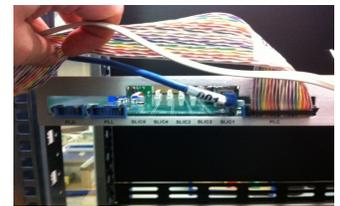
*Above photo set shows LTD020 termination device (left) ZX100 host PAGA processor (centre), note the blue RJ45 connection lead to LTD020 is extended from a standard ZX100 SLIC A subscriber line interface card (right).*
