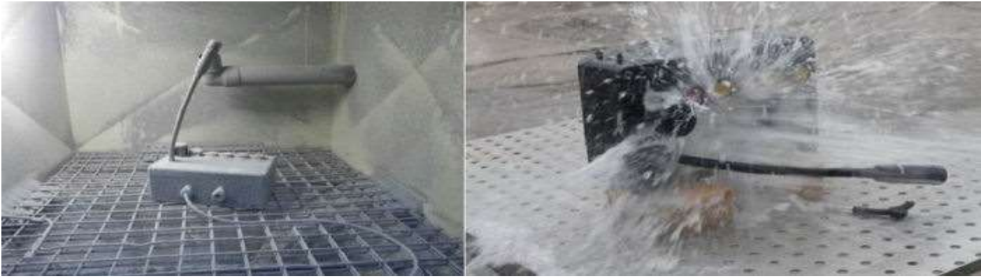
Zitel access unit undergoing independent ingress protection testing to IEC 60529
