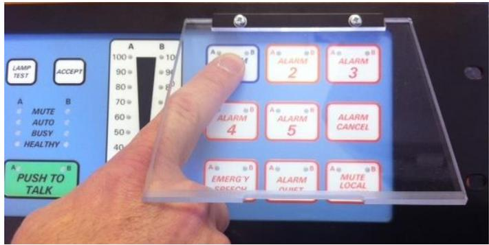
Critical control keys are guarded to prevent accidental operation. (note the cover guard material is stainless steel to eliminate static discharge risk)
