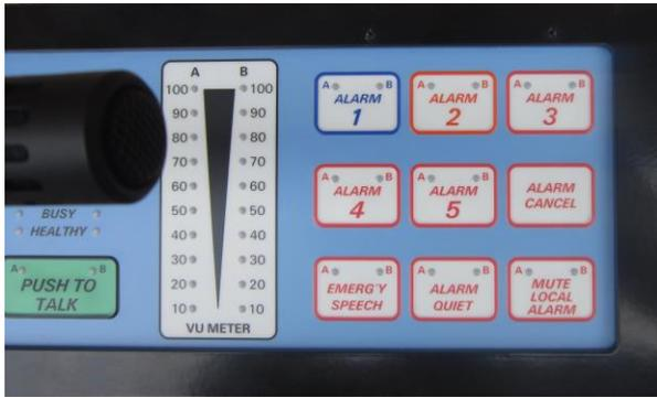
Dual VU meters aid efficient microphone technique ensuring consistent high quality speech broadcast.
