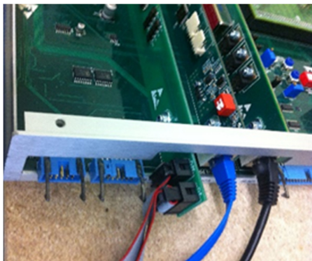
Photo shows the rear view ZX100 PAGA control unit with SLIC D installed.
