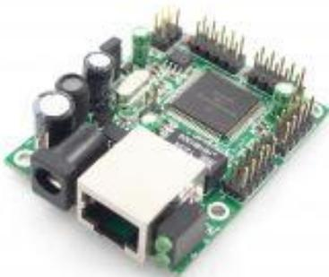
The ZDAENETIP42 is a flexible network device commonly used to provide interface between our central PAGA systems to Process Control Systems, ICSS or DCS.
