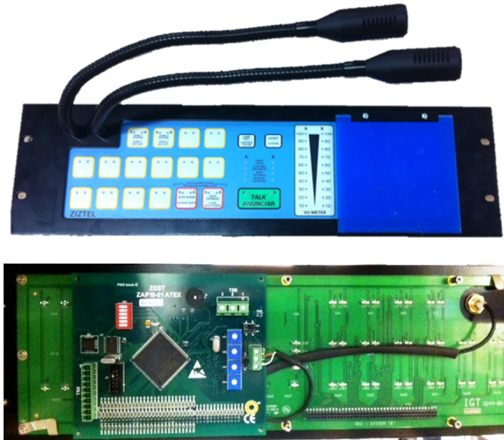
Photo shows ZAP10-01 Zitel transceiver installed on an AP100-01 access unit.
