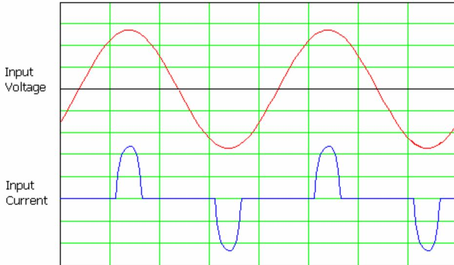
During times when the system is in quiescent and power demand is small the diode bridge connects the capacitor to the AC source when the voltage is near the peak, resulting in an abridged sinusoidal shaped current wave with current only flowing for about 1 to 2ms every half cycle. Although the current is nominally in phase with the voltage the distorted nature of the current waveform creates potential problems for the AC voltage supply.
