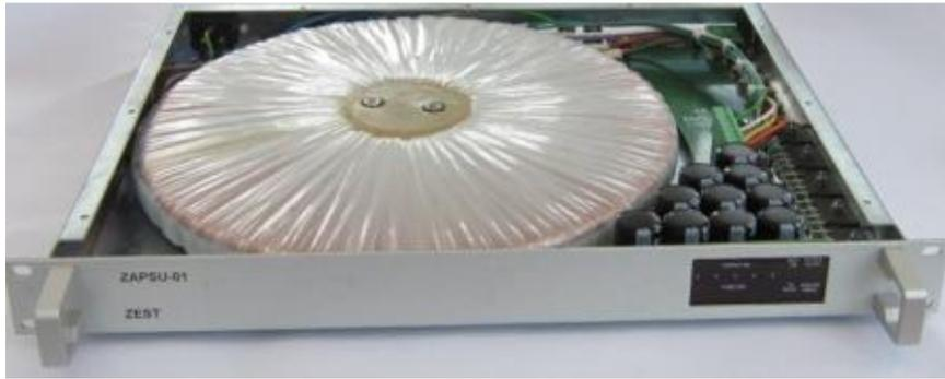
Zitel ZAPSU-01 power unit shown. This unit takes linear power supply design to its ultimate progression. There are 5x PSU units housed in a 1U 19-inch case to energise 4x on line and 1x standby 350 Watt amplifier modules with staged switch on to eliminate surge.
