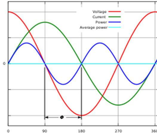
*Instantaneous and average power calculated from AC voltage and current with a zero power factor ( $\varphi = 90$ ,  $\cos \varphi = 0$ ).*
