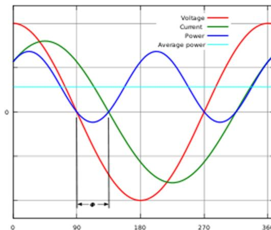
*Instantaneous and average power calculated from AC voltage and current with a lagging power factor ( $\varphi = 45$ ,  $\cos \varphi = 0.71$ ).*
